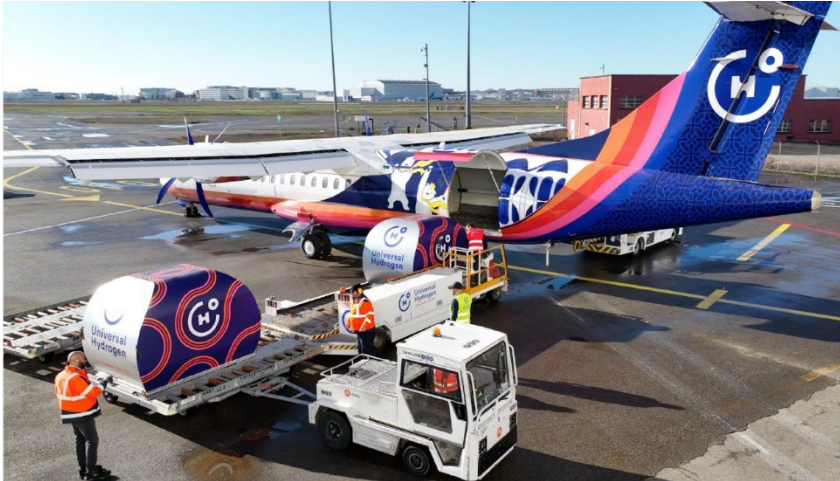
Figure 8 Hydrogen module exchange, technology demonstrator: Courtesy of Universal Hydrogen.
