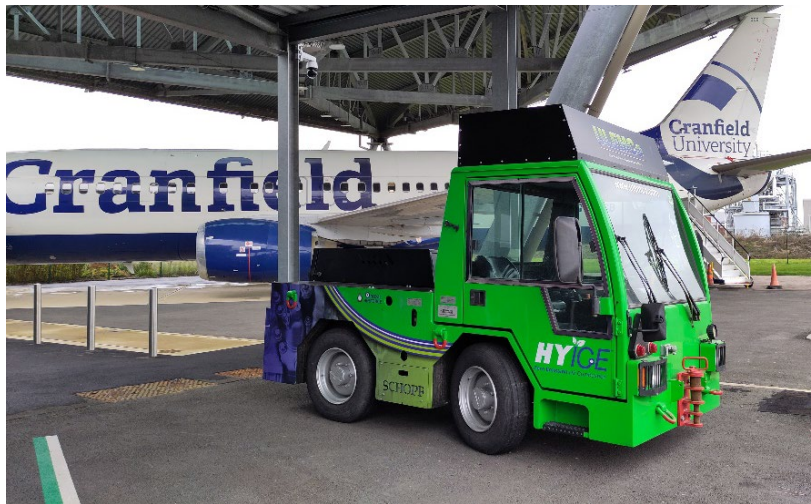
Figure 10. Hydrogen-powered aircraft tug being tested at Cranfield University. Courtesy of Cranfield University
