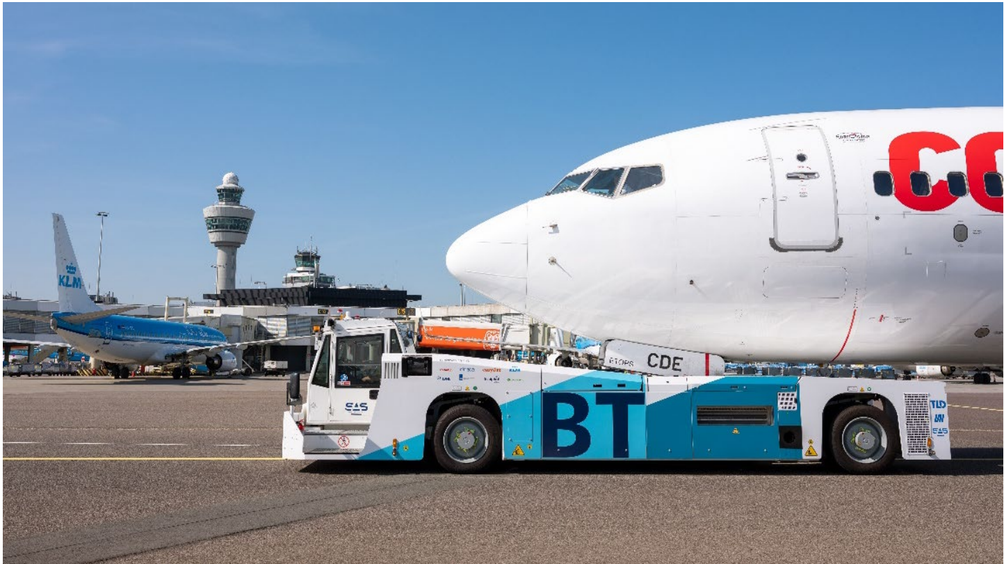
Figure 3. Taxibot in use at Schiphol Airport. Example of extended towed taxiing operations. Courtesy of Schiphol Group.
