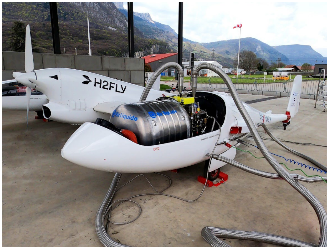
Figure 6. Liquid hydrogen refueling operations of the first-ever LH 2 -powered demonstrator flight. Courtesy of H2FLY.
